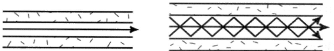
Figure 12. Left: a single mode fiber, only one mode can pass through the fiber. Right: a multimode fiber, more light can pass through the fiber. The light is captured in the core.
