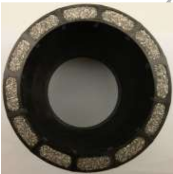
Figure 1: The regenerators' casing filled with magnetocaloric materials
