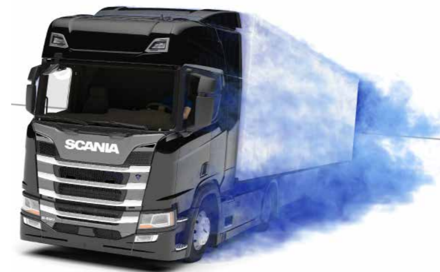
Above: Volume rendering of the instantaneous velocity magnitude on the leeward side of an R20 Highline truck at crosswind conditions (Source: Scania)
