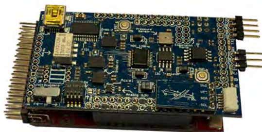
Figure 4.1: The controller board, with the inertial estimation board on top
