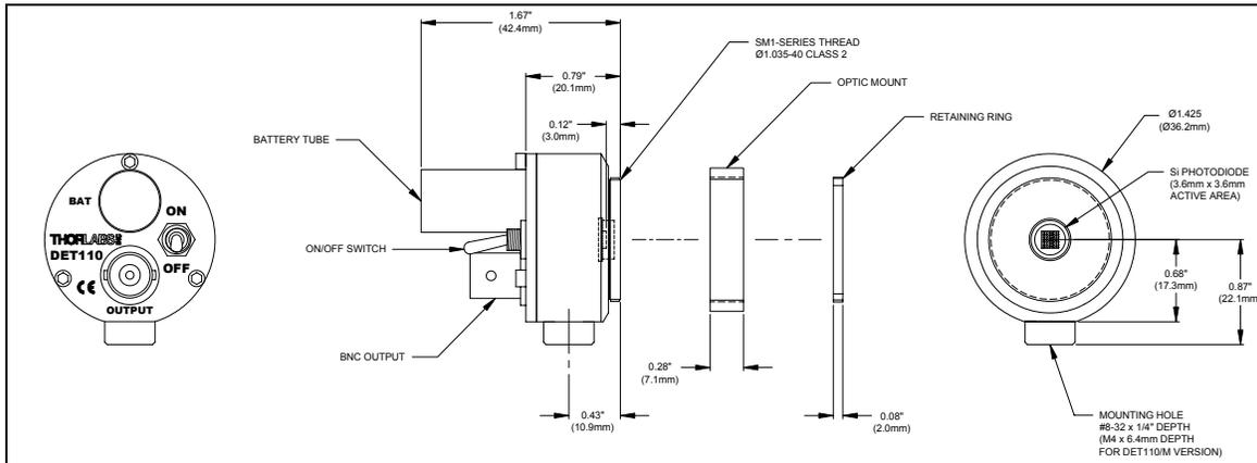
Figure 1. - Mechanical Dimensions
