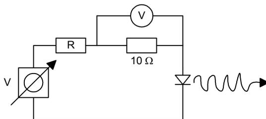
5. Switch on the voltmeter. Use the 2V DC range.
