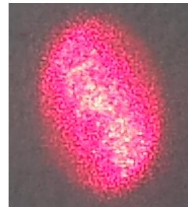
**Cause:** high degree of laser light coherence
