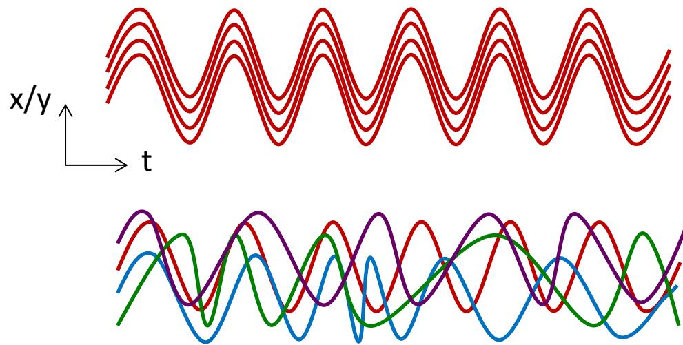
**Spatial coherence:** waves at two lateral points (along x/y direction)
