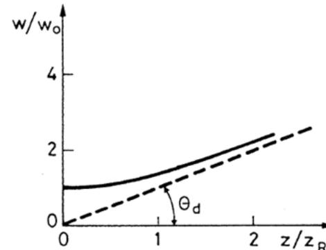
$$\text{Diffraction limited beam: } \theta_d = \beta \frac{\lambda}{D} \quad \text{with } \beta \approx 1$$
