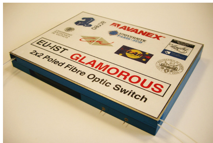
Figure 8.3. Final demonstrator of the Glamorous project. The package was designed by Avanex, one of the partners in the consortium. The interferometer was produced and tested by the author. This device has an optical bandwidth of 7 nm and V_{\pi} = 230 V [paper VI].
