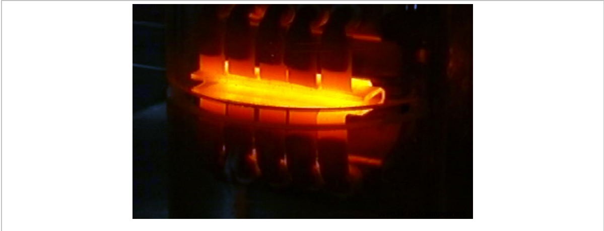
Figure 7.13. Oven used to pole the fiber for different time intervals. The oven is open at one side so that fibers can be quickly inserted and removed, and has a low temperature gradient in the hot zone.
