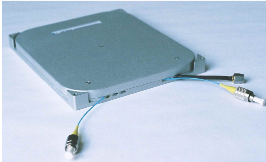
Figure 8.2. Optical modulator in new package as demonstrated at ECOC in September 2004 in Stockholm. A CW laser was coupled into the modulator, which was driven with the signal from a DVD player (~5 MHz). The modulated optical signal was detected with a photo diode and displayed on a TV screen to show the overall performance of the device. The two optical pigtailed and the SMA connector for electrical drive signal can be seen.
