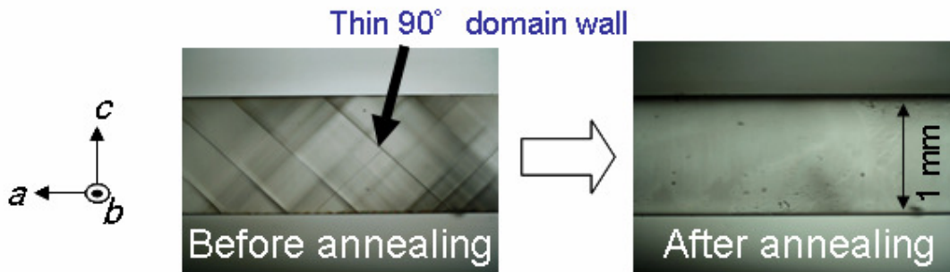
Figure 5-4-12. Removing unwanted domains in PPKN by annealing as a post-poling process.
