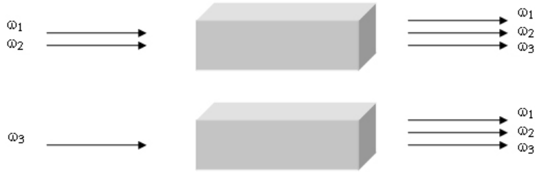
Figure 6.1. Two general non-linear processes; two incoming waves mixing, resulting in SHG, SFG, and DFG; or energy from one wave dividing between two generated output waves resulting in OPO and OPG.
