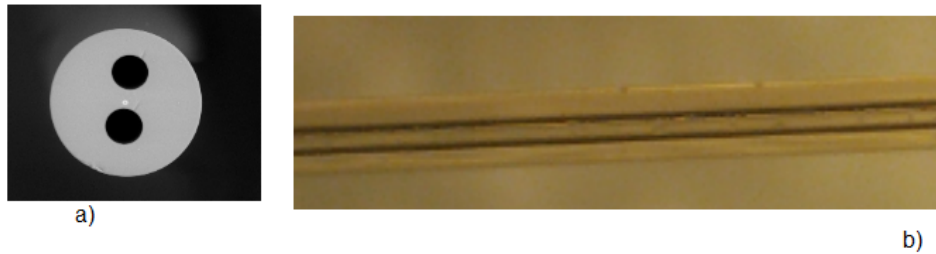
Figure 4: a) Front of a non-symmetric two-holes fiber [4]. b) The holes have a diameter of 27\mu m and a distance of 22.7\mu m . BiSn is seen inside the holes.
