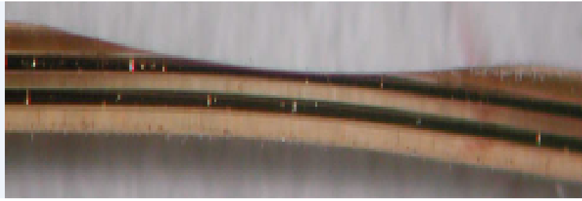
Figure 11: Coating and part of the cladding are removed. Here the fiber is very fragile.
