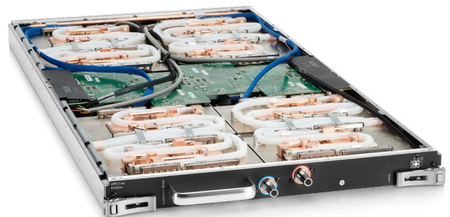
Above: The photo shows an HPE Grace Hopper Superchip board with two nodes. Each node contains four NVIDIA Superchips, each with a CPU and a GPU. The board is made by HPE using the NVIDIA Grace Hopper Superchips.
