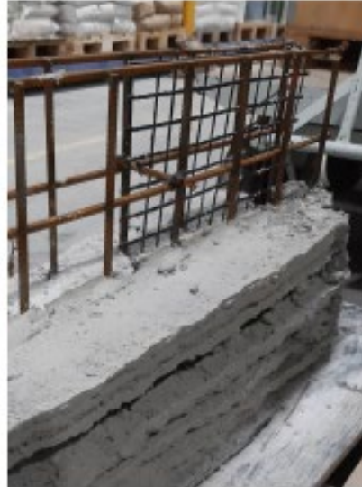
b) Printed wall, side view
