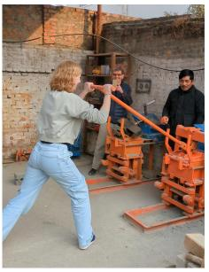
My project in Nepal focused on developing eco-friendly bricks with the goal of reducing cement usage while maintaining strength. Cement production is a significant source of CO2 emissions, so this initiative supports sustainable construction practices and aligns with the UN's Sustainable Development Goals. Additionally, cement is expensive, making it beneficial to reduce its use, especially in a developing country like Nepal.
