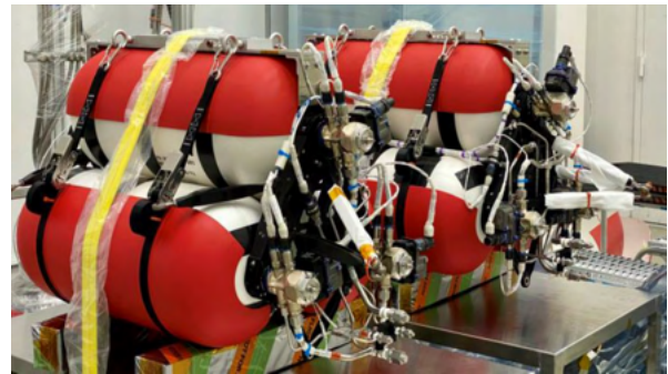
Fig. 3. Oxygen and nitrox bottle packs in the Crew Dragon [2]
