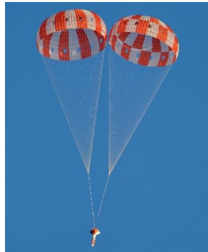
Fig. 11: Orion's two main parachutes inflated from a test
