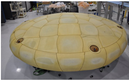
Fig. 10: Heat shield of Crew Dragon
