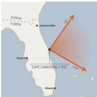
Fig. 1: Launch azimuth restrictions for KSC. Launch azimuth of 35^\circ results in an inclined orbit at around 57^\circ
