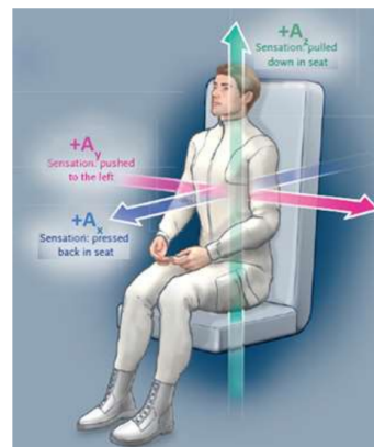
Fig. 9: Common XYZ Coordinate Frame for Translational Acceleration [22]
