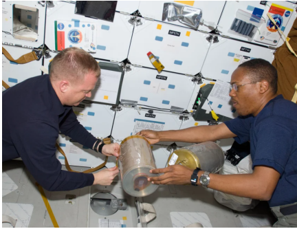
Fig. 3: Canister \text{LiOH} , used on space shuttle Discovery. A canister of approximately 0.014 m 3 can sustain \text{CO}_2 removal for 2 man for 2 days. Our design would include 2 of them.
