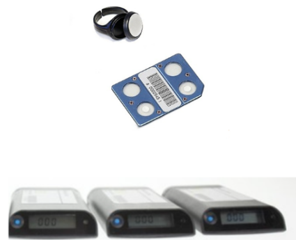
Fig. 8: Example devices that can be used on board, The example for the active device is European Crew Personal Active Dosimeter [12] and for a typical TL detector [2]
