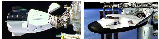
Fig. 8. Location of the docking system at the front for the Crew Dragon (left) and at the back for the Dream Chaser (right).
