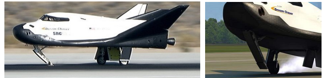
Fig. 5. Dream Chaser landing method as an airplane (left), with a front skid to facilitate this (right)
