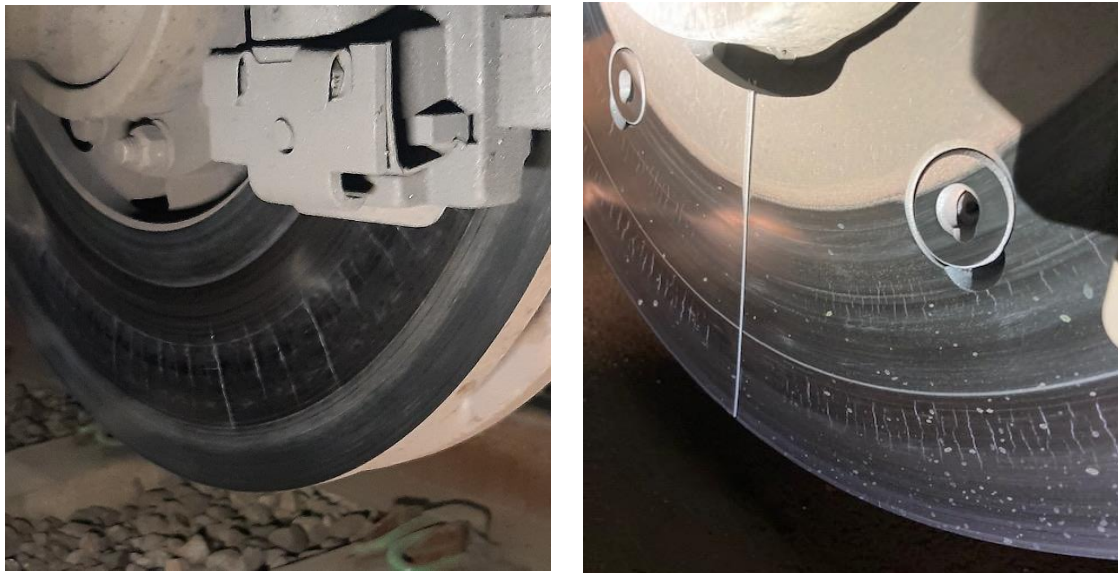
Figure 1. Cracks on non-segmented disc (left) and segmented disc (right) for long-term usage.
