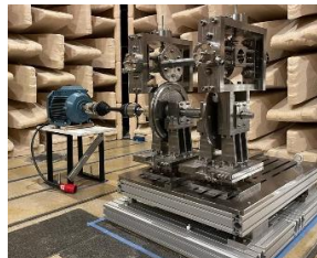
Figure 1. Roller Rig mounted at the MWL lab at KTH.
