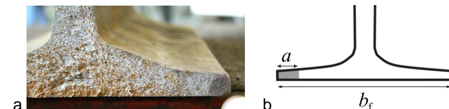
Figure 1. a) Rail break from foot crack (picture Anders Frick) and b) definition of idealised foot crack of size a .
