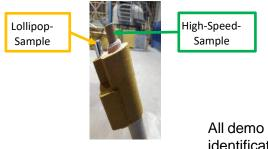
Measuring equipment was set up in laboratory successfully. Combination sampler of high-speed sampling and conventional Lollipop sampling was developed and tested successfully.
