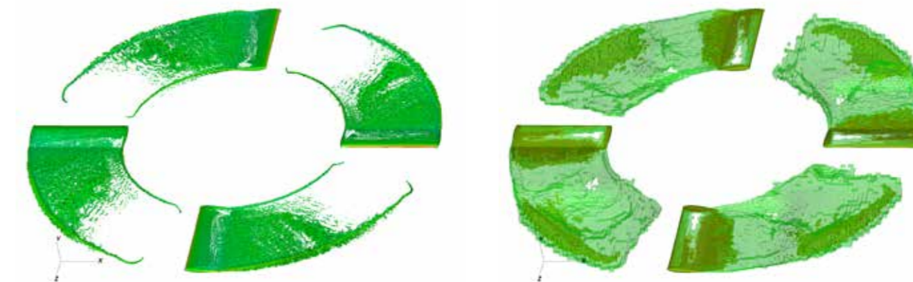
Below: "Toy" rotor – (left) vortical structures identified using the lambda2 criterion and (right) regions of higher refinement computed dynamically by ARM
