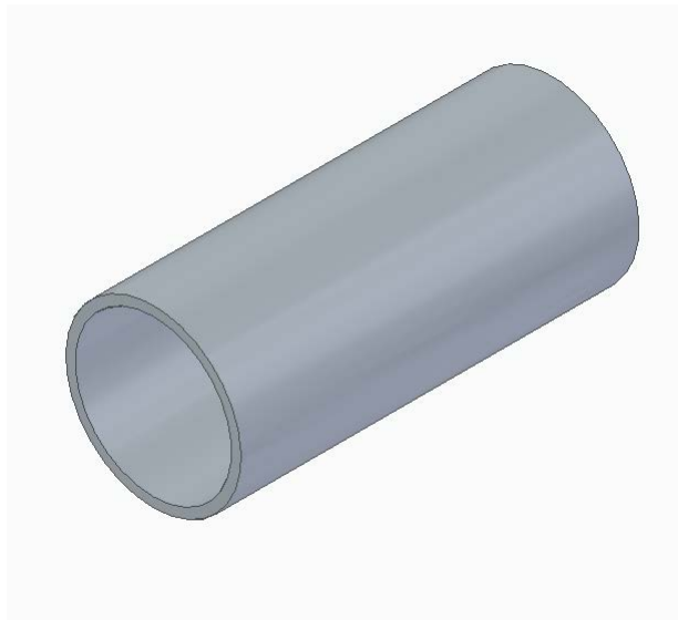
Figure .11. Cylinder for US sensor created with Solid Edge.
