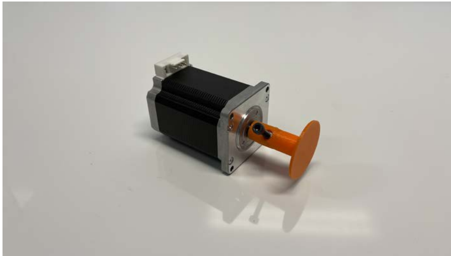
Figure 3.4. Sanyo Denki 103H7823-1740 Stepper motor with 3D-printed axle attachment. Photo taken at KTH mechatronics lab.
