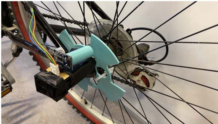
Figure 3.2. Back wheel sensor system. Photo taken at KTH mechatronics lab.
