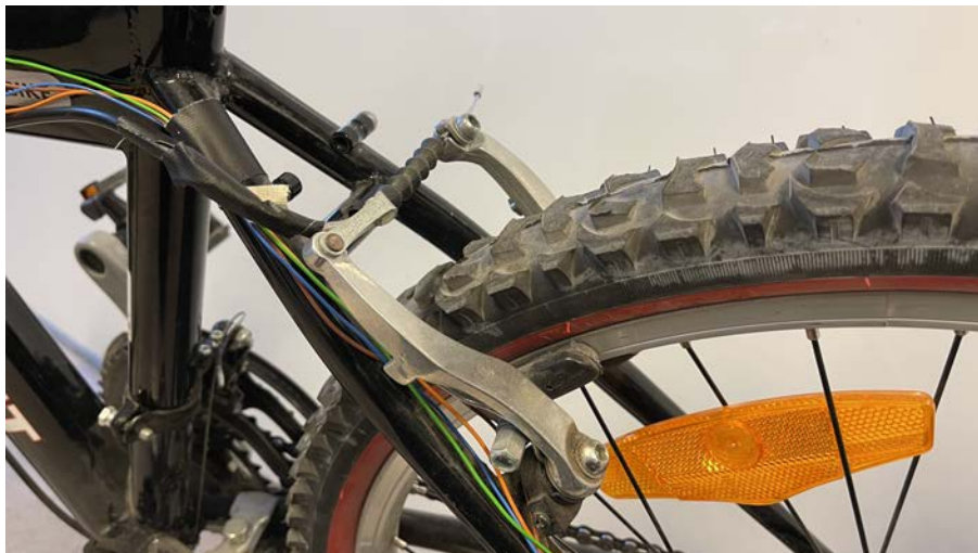
Figure 2.1. Back wheel V-brake. Photo taken at KTH mechatronics lab.
