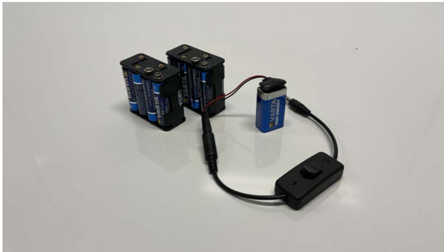
Figure 3.6. 16 AA batteries and a 9V battery with a switch. Photo taken at KTH mechatronics lab.
