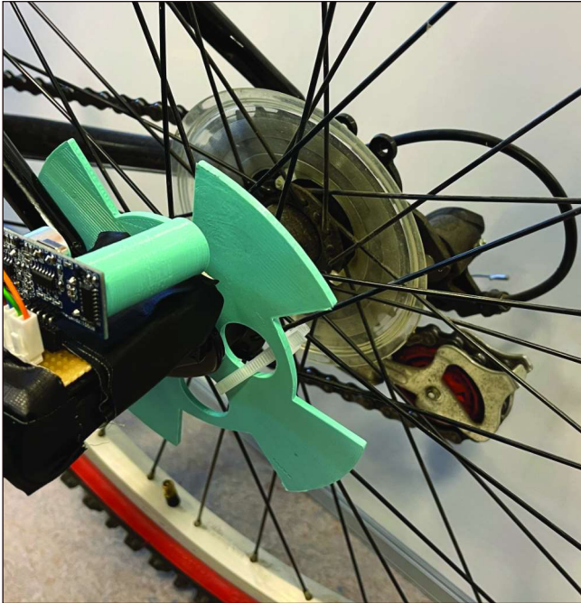
Ultra sonic sensor detects if the wheel is spinning or not.
