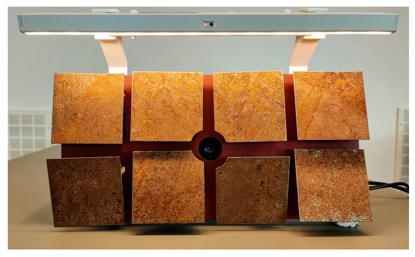
The final construction. The pixels rotate in order to reflect different amounts of light from the lamp, thus mirroring the captured image.
