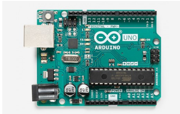
Figure 2.1. Arduino Uno Rev3 [4].
