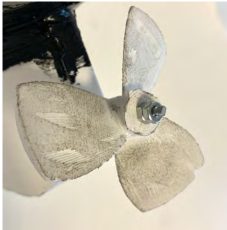
Figure 3.3: A propeller and its connection to the axle. Taken by authors.
