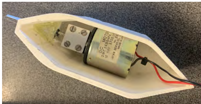
Figure 3.2: Gondola with motor and propeller axle. Taken by authors.
