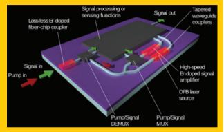
lasers are reviewed and current and future potential applications are explored. The vision of integrating such Er-doped gain devices with other, passive materials platforms, such as silicon photonics, is discussed.
