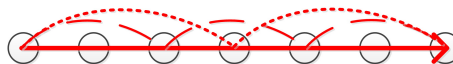
Figure 6: Simulated network topology with a single flow. The transmission range is set to 50 m, 100 m, and 150 m in different simulation runs to produce paths with two, three, and six hops, respectively.
