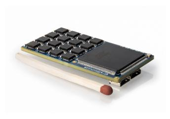
Fig. 1. In-house developed inertial sensor array with 288 sensing elements. The array is built out of 32 InvenSense MPU9150 sensor chips.
